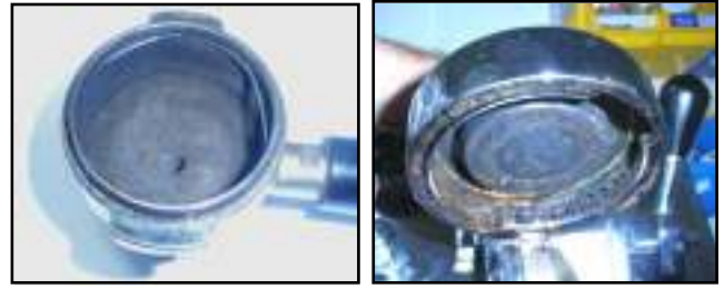
Coffee oils build up on machine surfaces and become rancid.
